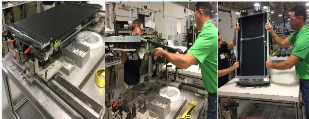
Bosch Rexroth desires that students design a new assembly fixture that resolves the previously mentioned problems. There is particular interest in a rotary assembly fixture which will allow an operator to work on both sides of the HQ2/U unit without having to remove it from the fixture.
